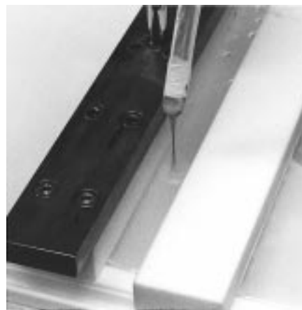
Figure 3. Removal of poly(BAD) from the surface of the Langmuir trough. The polymer comes off the subphase in self-supporting, elastic sheets which easily draw down to fibers.
